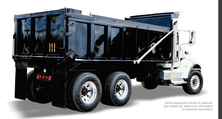
FEATURES VERTICAL SIDE BRACING AND RUGGED TOP RAILING CONTINUOUSLY WELDED FOR MAXIMUM STRENGTH
